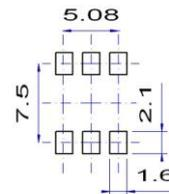
**Do not design any conductive path between the pattern**
