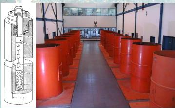
Today's autoclaves have dimensions, up to a height of several 10 meters and one or more meters in diameter. The inner conditions have stayed the same for more than 100 years, pressure of 2000 bars and temperatures of 370°C. Electric heat provide the right temperature and the growing time runs from several weeks up to one year, depending on
