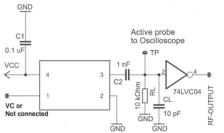
Test circuit for CMOS
