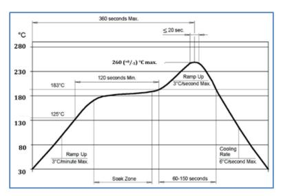
Maximum Reflow Condition in accordance with JEDEC STD-020C
