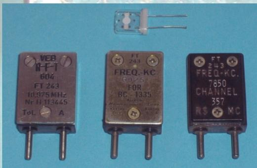
An important period for speeding up progress of the crystal development and production was the World War II and the following Cold War. Crystals were used for the communication systems and radar. Later on the Global Positioning System was built. All this needed a very precise time keeping. One of the first mass produced crystals was the so named "Channel crystal" for communication. It had standard dimensions and was produced from different factories for the same use.
