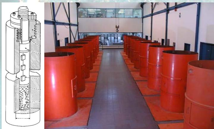
Today's autoclaves have much greater dimensions, up to a height of several 10 meters and one or more meters in diameter. The inner conditions have stayed the same for more than 100 years, pressure of 2000 bars and temperatures of 370°C. Electric heat provide the right temperature and the growing time runs from several weeks up to one year, depending on
